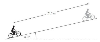
As the cyclist pedals, there is a constant forward force on the bicycle of  $150 \, \text{N}$ . The cyclist travels  $215 \, \text{m}$  along the slope.
