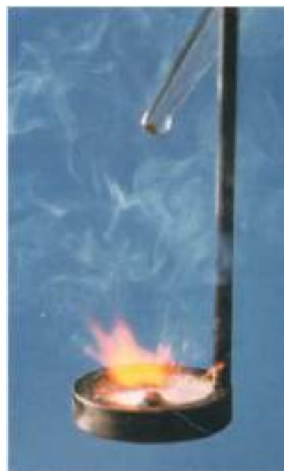
Sodium reacts with water vigorously and produces hydrogen gas which burns instantly
