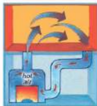
Warm-air heating system
