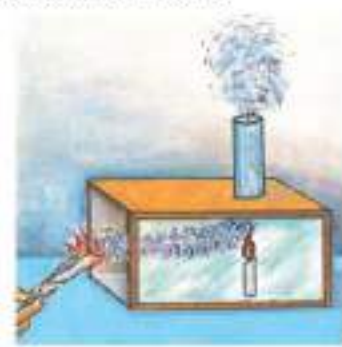
Figure 7.8 Demonstration of convection currents in air.
