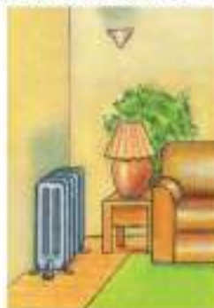
Figure 7.7 Black marks seen on the wall above a lamp or a radiator.
