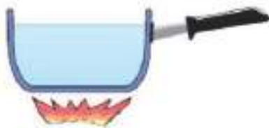
Figure 7.2 Plastic handles prevent heat conduction
