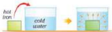
Figure 6.2 When a hot iron piece of iron is in contact with cold water thermal energy is transferred from the iron to the water.
