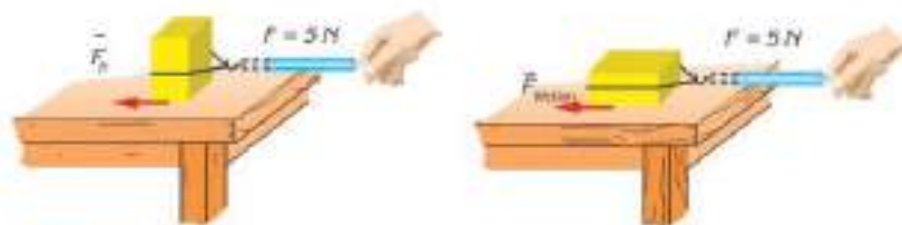
Figure 4.10 Frictional force doesn't depend on the area of the rubbing surfaces for objects made of the same material.
