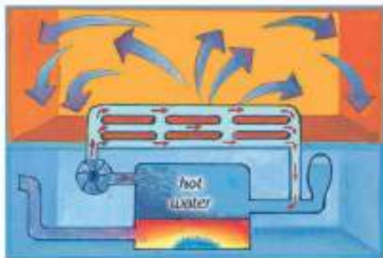
Hot-water heating system
