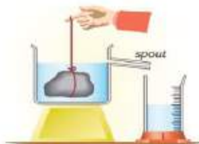
Figure 2.7 using overflow can
