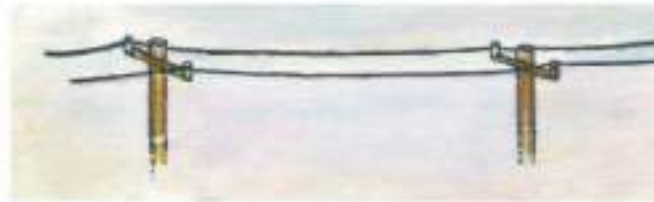
Telephone cables contract in winter.
