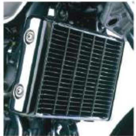
Car and motorcycle radiators are painted black to radiate away heat as quickly as possible.
